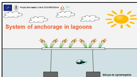
**Figure 3:** GFF anchorage to the bottom by means of ballasts.
