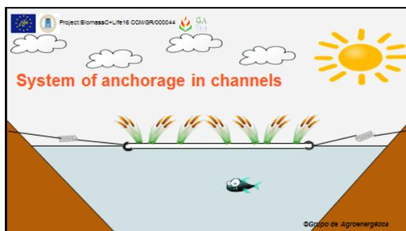
**Figure 4:** GFF anchorage to the banks.
