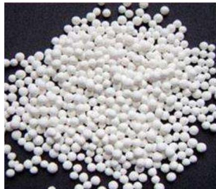
Despite the fact this material was used during the 2018 plantations, VOLTERRA does not recommend it as the disadvantages are higher than the advantages. Nevertheless, if used we advise an EPS density of at least 30 kg/m<sup>3</sup>. Less than that
